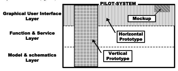
Figure 4: Differences among mock-up, horizontal prototype, vertical prototype and the pilot-system from an ANSI/SPARC three layer perspective.
